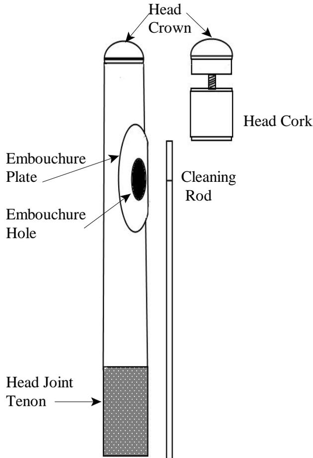
Outside of the normal pad and cork problems which can afflict all woodwinds, there are three main types of problems which can affect flutes. One problem area is the head joint. There are three potential problems with the head joint: the tenon, the embouchure plate, and the head cork.
