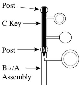
Notice how the hinge-pivot (solid black object) passes through the top post, through the hinge tube of the C key, threads into the second post, and the point rests in an appropriately shaped opening in the key assembly which has the B $\flat$  and A keys on it (open hole flutes also have the G key on this assembly.)
