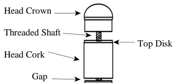
The problems which can result from a gap between the head cork and the bottom of the assembly mainly affect the upper notes, high C and above. They either have a bad tone, sound the incorrect pitch with the correct fingering, or are badly out of tune with the rest of the instrument. Very often this can be resolved by removing the head cork assembly, tightening the top disk, and reinserting the assembly into the head joint.
